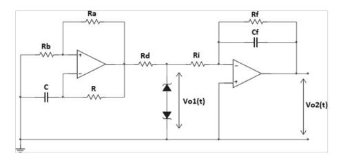
dove  $R_a$ =1 k $\Omega$ , R=8,2 k $\Omega$ , C=7,5 nF,  $R_a$ =2 k $\Omega$  e  $R_b$ =7 k $\Omega$ .
